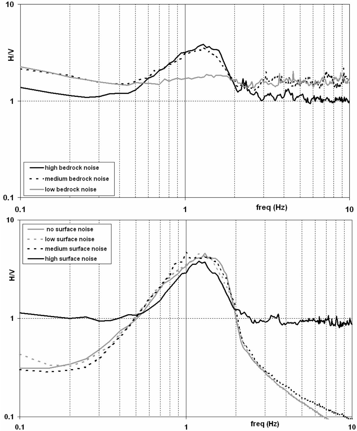
**Fig. 5 (top) effect due to the input noise level; (bottom) effect on HVSR when the unfiltered noise at the surface (e.g., wind) increases.**
