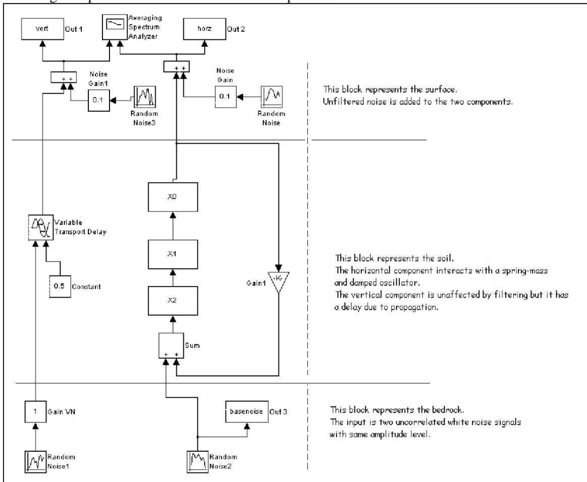
**Fig. 4 Matlab Simulink block model: uncorrelated Gaussian white noise is processed by a filter simulating a spring-mass-damper device.**
