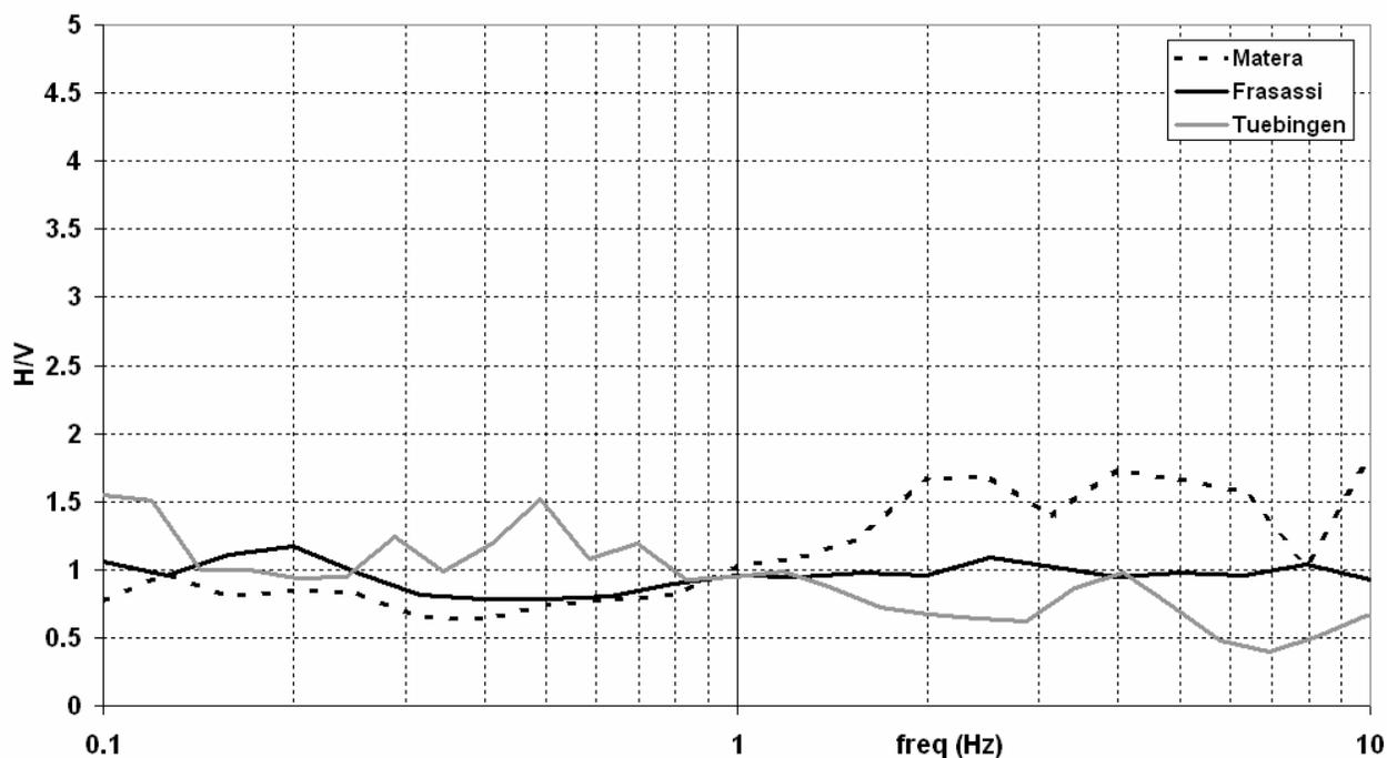
Fig. 2. H/V by noise at bedrock: Frasassi, Italy (cave at 1000 m depth); Tuebingen, Germany (borehole at 100 m below the surface); Matera, Italy (cave at 10 m depth).
