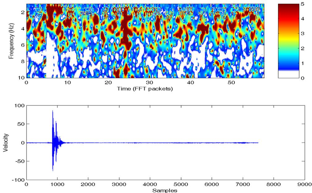
**Fig. 3. Moving window HVSR during a SASW test. The main pulse, composed by Rayleigh waves, shows a strong de-amplification at frequencies higher than the fundamental mode.**
