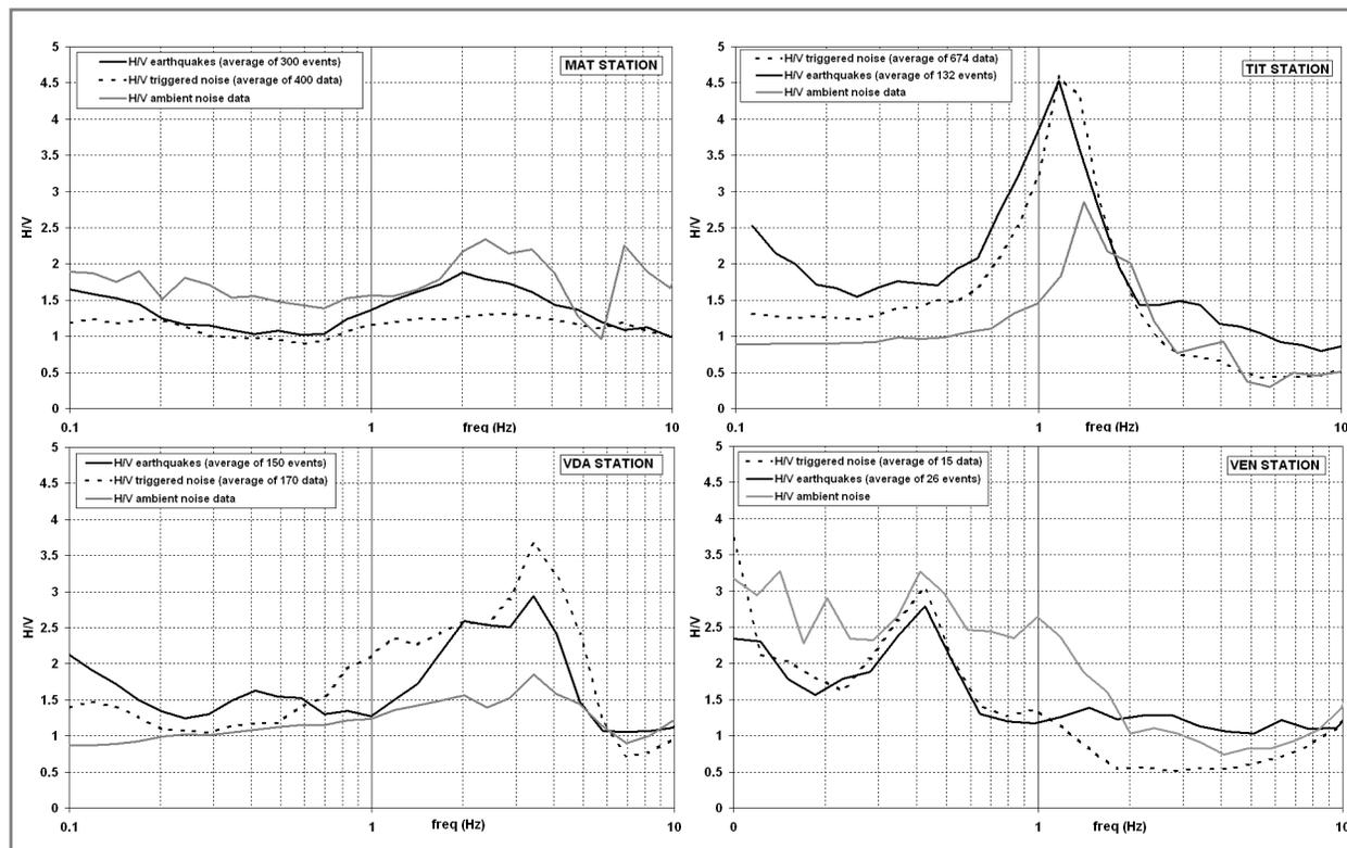
Fig. 1. H/V by earthquakes, triggered noise and microtremors obtained for the four stations.
